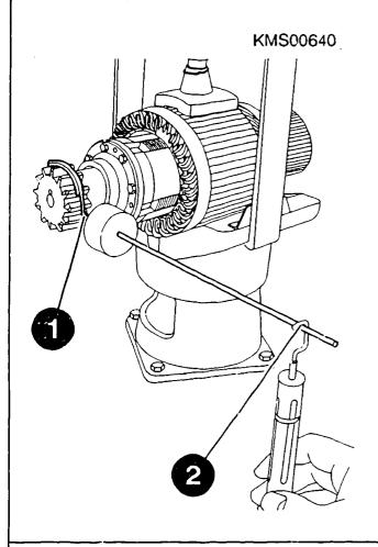
Checking axial play of gear shaft
